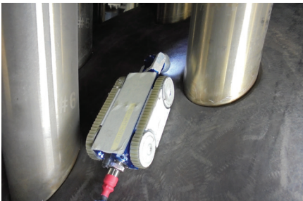
Visual inspection services for penetration pipes of reactor head
